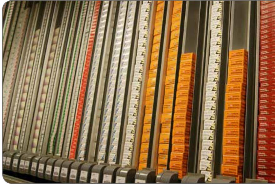
A Fastmover Channel consists of a vertical channel with an automatic dispensing unit. The standard channel lengths are 1200, 1600, 1800, 2000 or 2200mm. Other lengths are available. The width can be chosen and adjusted to the selected package width. The FastMover channels can be controlled by an existing robot or by independent operating software.
